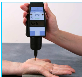
The Prod (0.5N -25N) in use on the thumb
