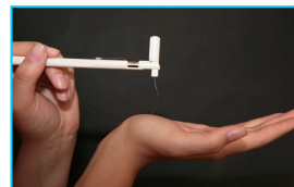
von Frey filaments are often used to measure mechanical thresholds in rats and mice as well as for identification of allodynia in larger species
