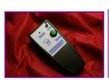
The systems are operated from a two channel handset; one channel applies the stimulus and the other resets the system for the next test. Threshold temperature is recorded automatically on the digital display on the band and is retained until the "status" button on the handset is pressed. The system is failsafe; the stimulus is removed if the infra-red signal is lost. There is also an electronic safety cut-out in the system if a preset temperature is exceeded.
