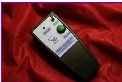
The system is operated from a two channel handset; one channel applies the stimulus and the other resets the system for the next test. Threshold force is recorded automatically on the digital display and is retained until the "status" button on the handset is pressed. The system is failsafe: the stimulus is removed if the infra-red signal is lost, and the maximum force achievable is limited by the air pressure in the pre-charge cylinder.
