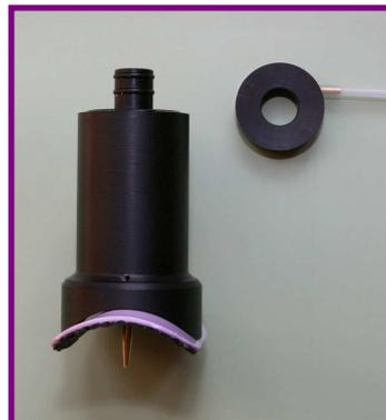
The mechanical actuator has a rolling diaphragm to ensure low friction and a “donut” O ring connection to the pressure line. This is designed to pull away without damage to the system if the subject becomes excitable. The standard pin diameter for large animals is 1mm. Other sizes, and a three pin configuration are also available on request. The actuator is supplied with mounting straps and boots and a dummy set for the contra-lateral limb.
