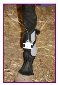
Our range of limb-mounted pneumatic actuators for mechanical threshold testing are light, low-friction and silent in operation.
