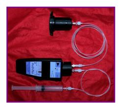
Each actuator set is supplied with a mounting boot, strap and buckle for the species being tested. Single and three pin geometries are available, with force ranges from 0.5 -25N. Every kit is suplied with a dummy fitting for the contra-lateral limb and quick-release "donut" fittings for pneumatic connection, designed to disconnect without damage in the event of unexpected sudden movement.
